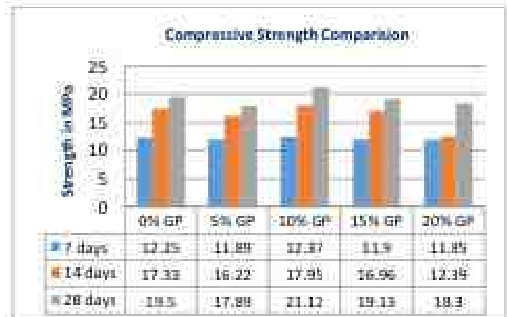
FIG1. Comparison between Compressive strength at 7days, 14 days & 28 days with 0%, 5%, 10%, 15 % & 20% replacement of cement by waste glass powder in concrete.
